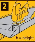
If required trim Threshold Ramp with a Jig-saw to suit.
