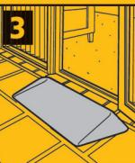
Simply lay in place or fix permanently with builders adhesive.
